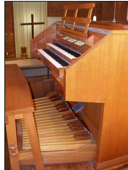
The console cabinet, pedalboard, casework, bellows, wooden pipes, windchests and electro-pneumatic actions were all made by Pogson, while the metal pipes were supplied by George Fincham & Sons, of Melbourne. The keyboards, key contacts, stopkey units and chest electro-magnets were supplied by Kimber-Allen, of Swanley, Kent, UK, while the electro-magnets for the console relays were made
